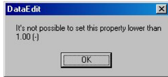
Figure 6 Example of warning message for a situation where the input parameter P is outside of the validated limits (hard limits) of the formula
