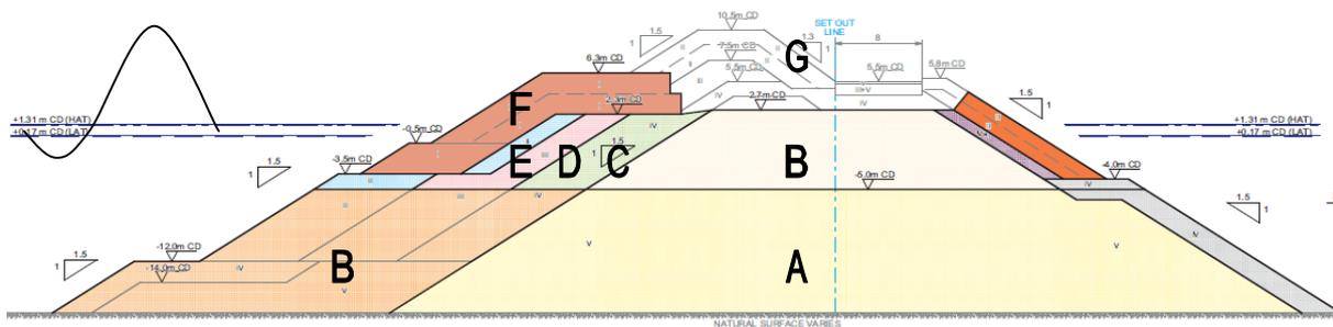
Figure 3. Typical Breakwater Cross Section, Construction Phases A to G shown
