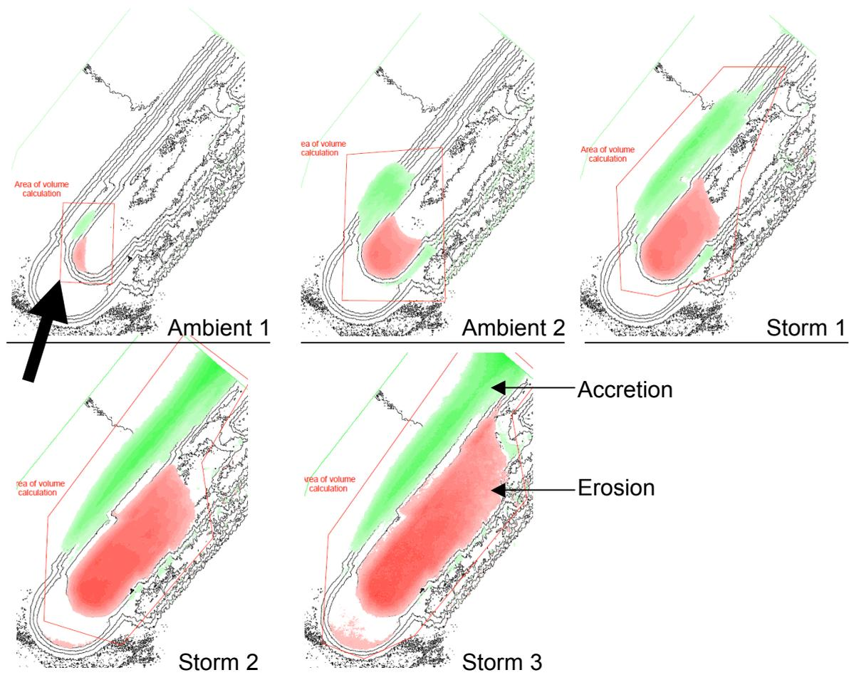
Figure 8. Damage Evolution, Causeway.
