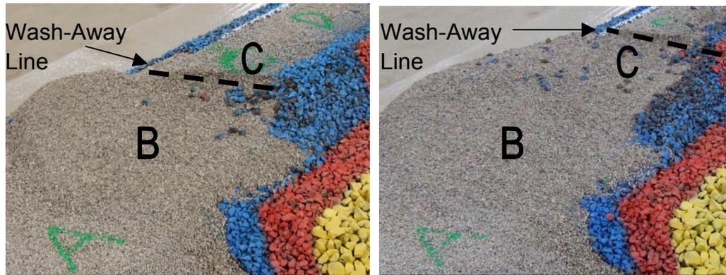
Figure 9. Core loss undermining armour layer, Trunk - Phase B and C.
