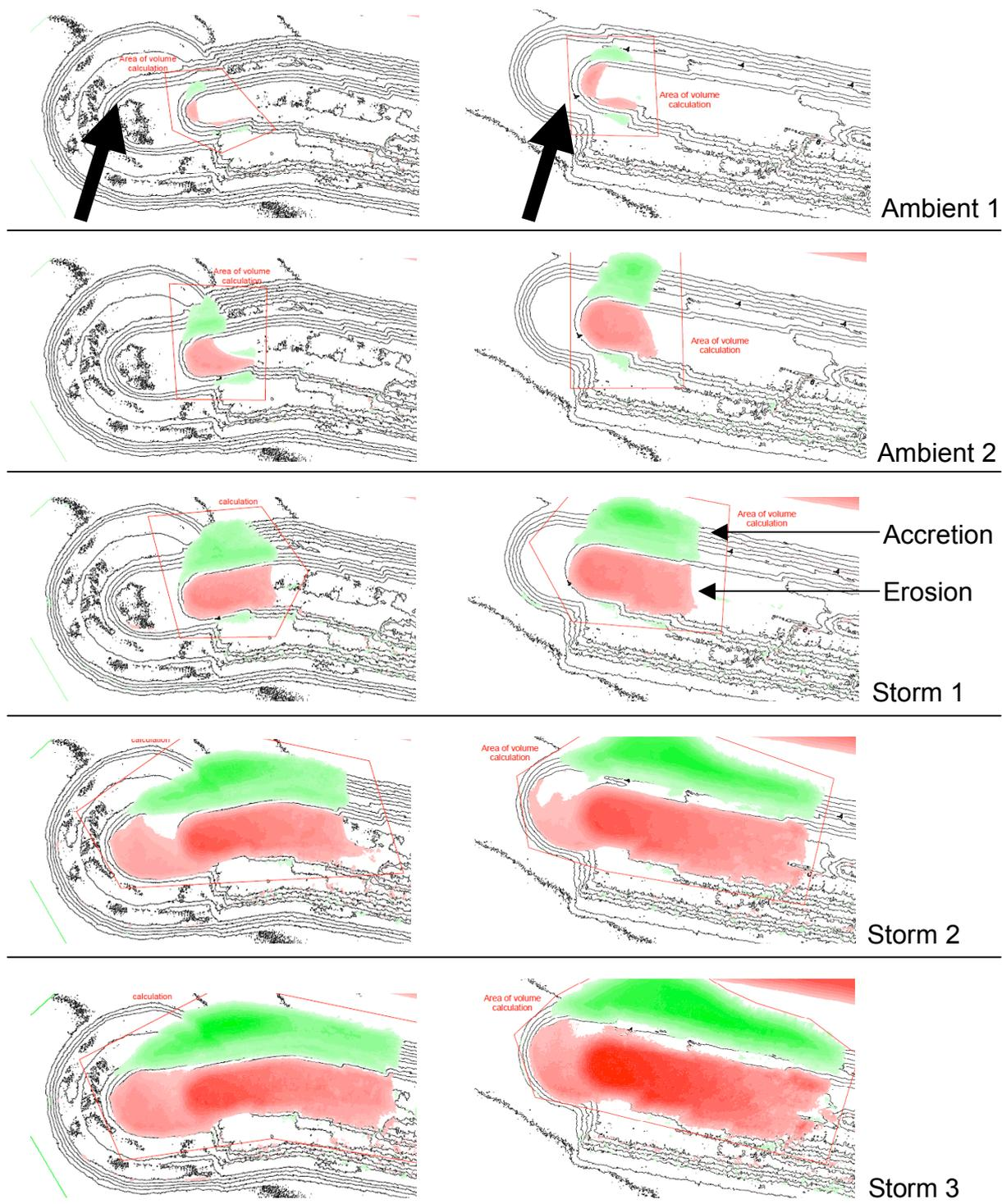
Figure 7. Damage Evolution, Roundhead (left), Trunk (right).
