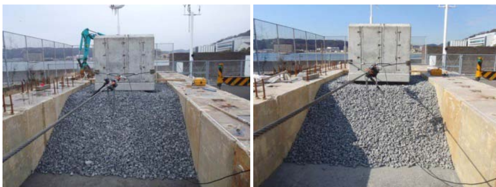
Photo 7. Initial state (left: Ratio of Joint flow Scour 30%, right Ratio of Overflow Scour 20%)
