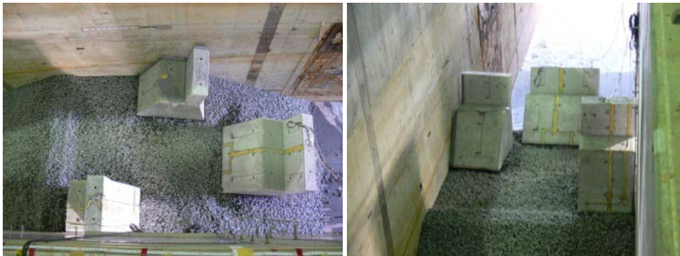
Photo 5. State of breakwater After Experiments (case2 trial 3)
