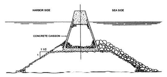
Figure 2: Sample detail of a composite breakwater
