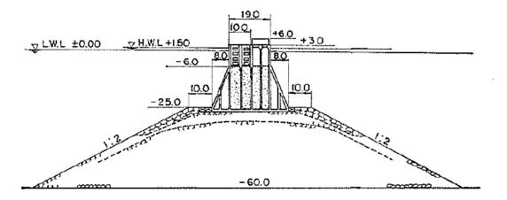
Figure 5: Originally proposed cross section of Kamaishi Breakwater
