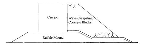
Figure 3: Geometry of wave dissipating concrete blocks against composite breakwaters (Source: Proceeding of 25th Conference on Coastal Engineering, Orlando, Florida, 1996)
