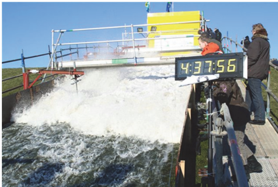
Figure 4.34 Release of a large overtopping wave volume
