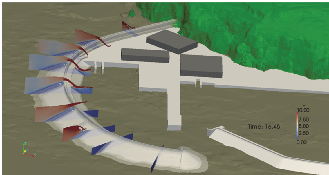
Figure 4.25: Numerical modelling results using the NS solver IHFOAM for the harbour of Laredo (Spain). The geometries of the bed, the rubble mound breakwater and the harbour quay walls are shown. At several sections along the breakwater, the simulated wave overtopping (i.e. the free surface configuration of the overtopping waves) has been visualised in 2D slices, to illustrate the complex and highly 3D wave interaction with the breakwater. Courtesy of J.L. Lara
