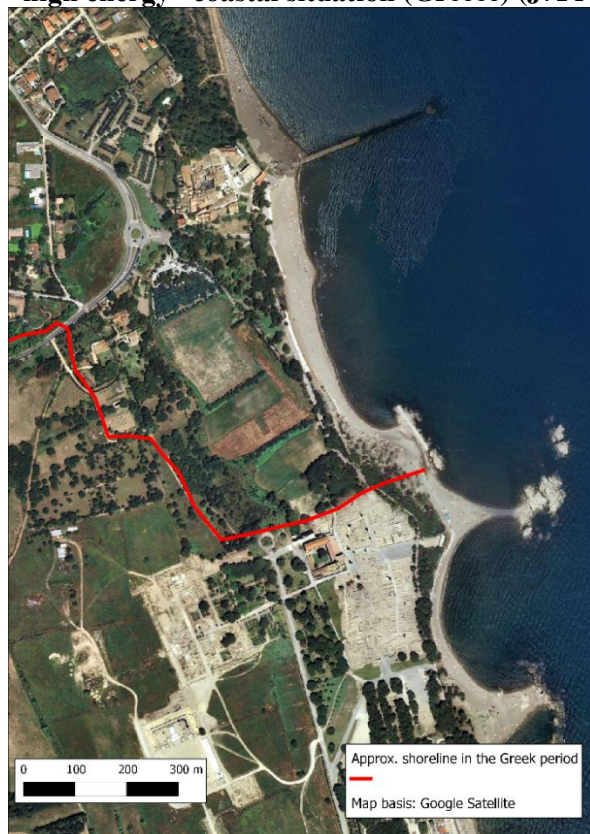
Fig. 2: The ancient harbour of Ampourias in Spain, with a silted harbour basin from the Greek period (red line) and remains of an eroded harbour basin from the Roman period to its east (J. Preiser-Kapeller, 2014)
