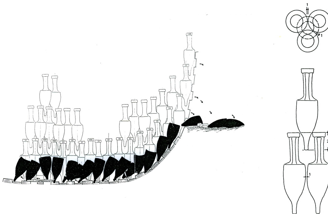
Figure 2: Theoretical reconstruction of the amphorae stowinf in the “Madrague de Giens” (Pomey 1997: p 149)
