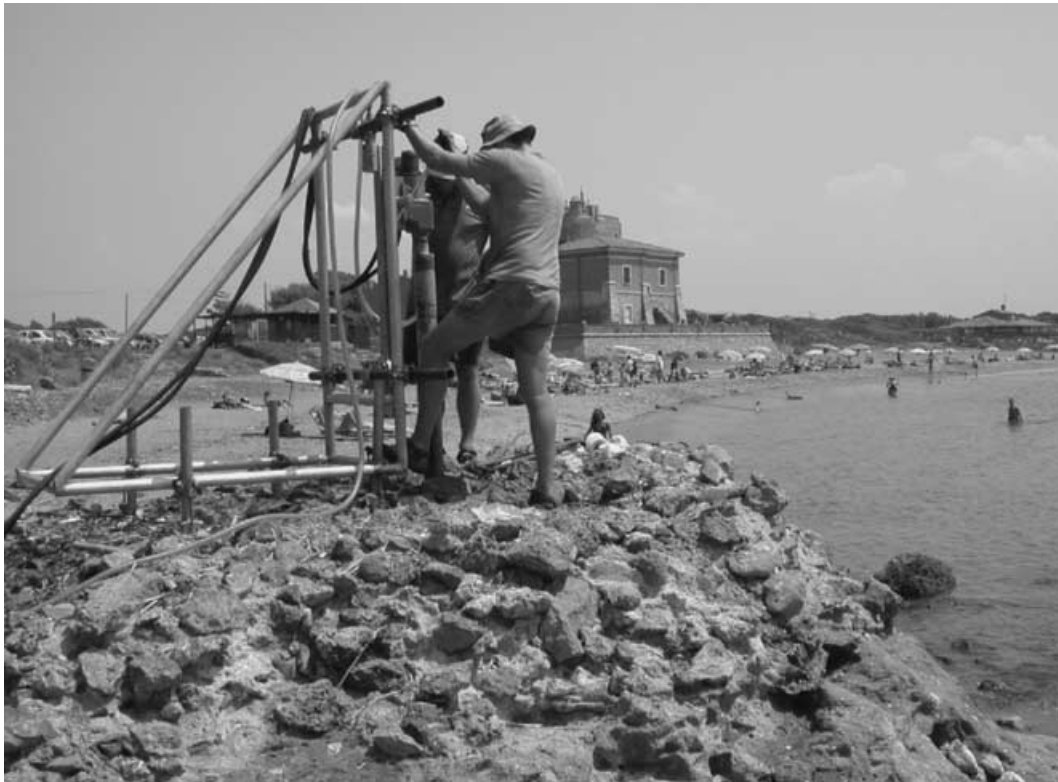
Figure 8. Coring device and frame in use at Cosa, Pier 1.
