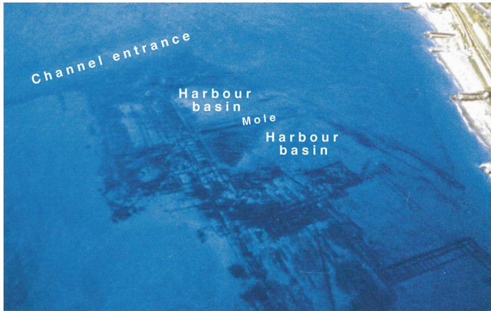
Harbors and ports, ancient, Figure 7 Pozzuoli's drowned harbor remains presently ~10 m below mean sea level. The site lies inside a caldera, where shoreline mobility is attributed to volcanism and faulting (Photograph: Centre Jean Bérard, Naples).
