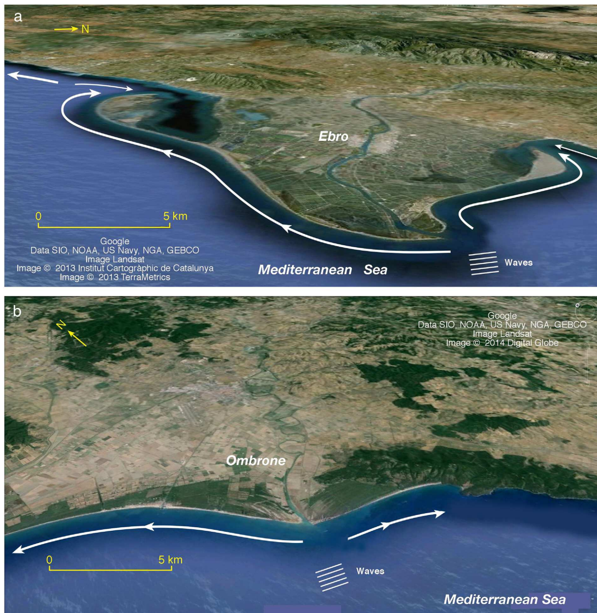
Fig. 15. The Ebro and Ombrone river deltas. These morphometrically relatively symmetrical deltas are characterised by divergent drift from the mouth following a pattern of progradation wherein delta growth has occurred to face the dominant wave direction.
