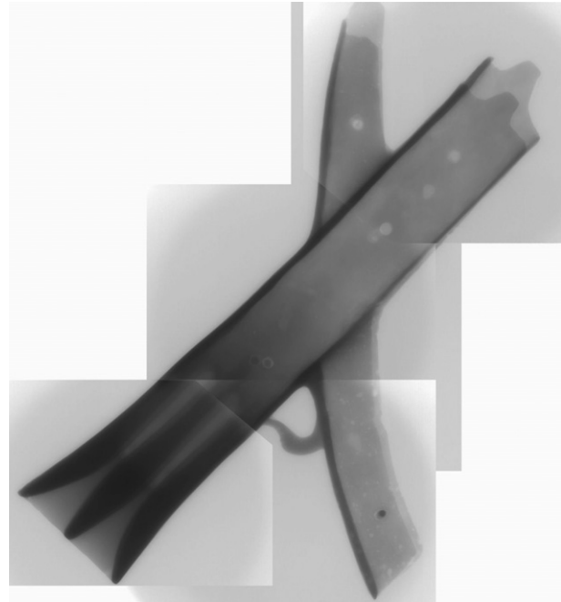
Figure 11. Composite radiograph of the ram. This is a positive image so that thicker metal is darker. (Crown copyright)
