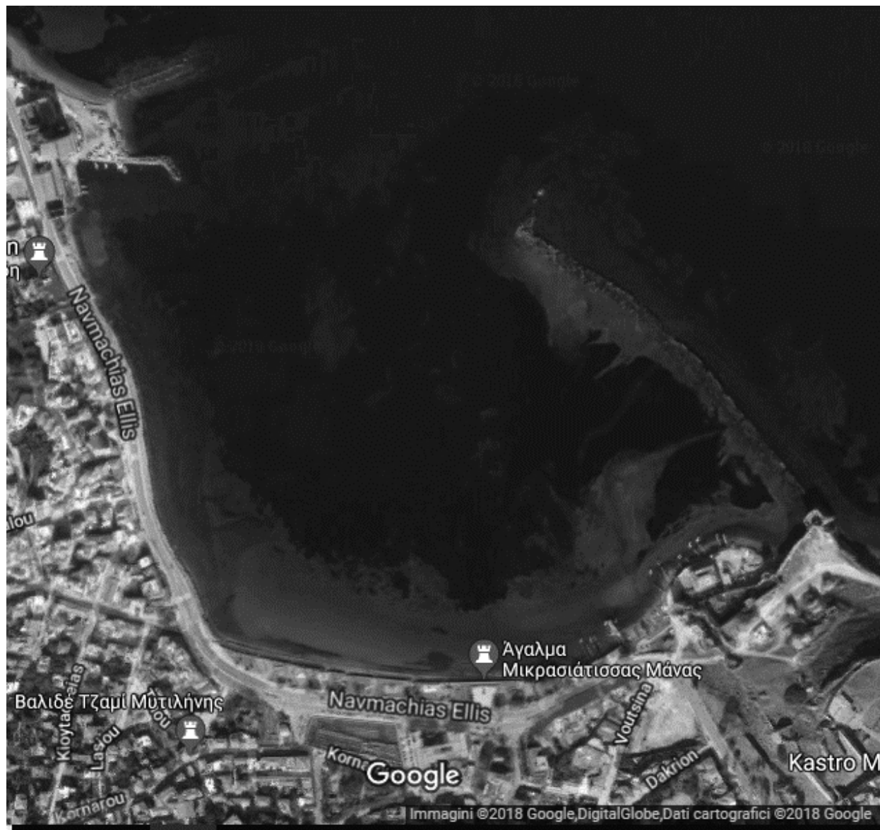
Figure 4.7. Satellite image of the commercial harbour of Mytilene, on the island of Lesbos (n° 115). Under the water it is possible to notice the remains of the southern and northern breakwaters which were extensions of the city-walls. Google Earth.
