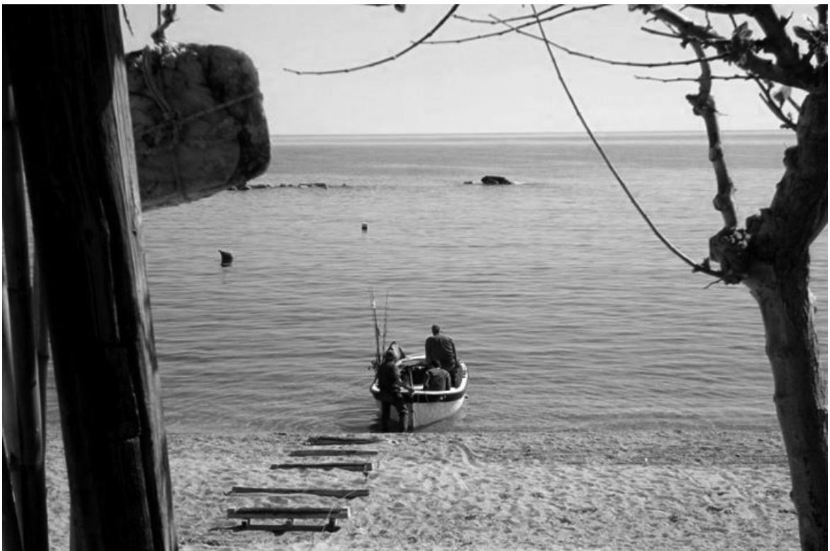
Figure 2.10. Traditional system used for hauling boats onto shore: wooden beams for hauling in the boats. Palizzi Marina (RC), Italy.
