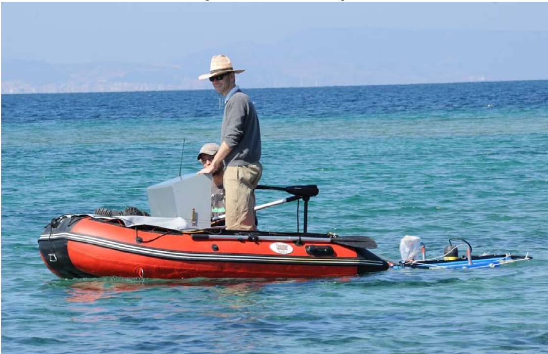
Fig: Marine seismic/acoustic reflection acquisition system, used for the Kane survey
