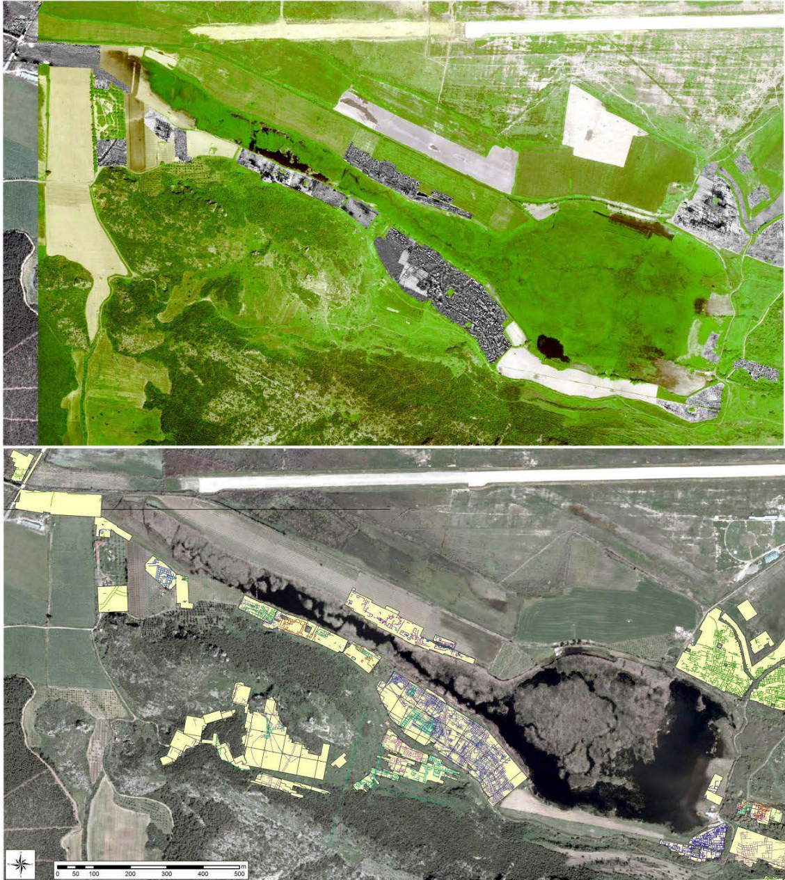
Fig. 3: Top: Results of the GPR surveys surrounding the harbour and harbour canal in Ephesos (black: high amplitudes - reflective, white: low amplitudes - absorbing). Bottom: Archaeological interpretation
