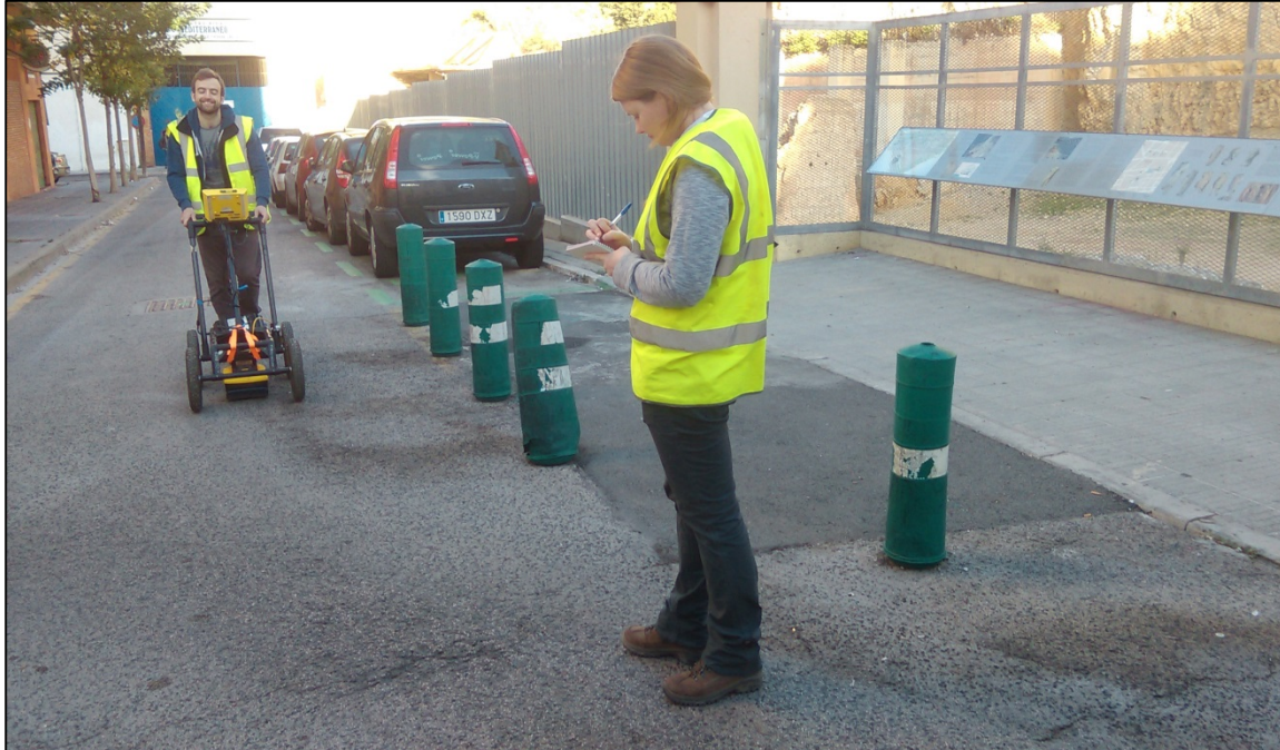
Fig: GPR survey with a 500MHz antenna being conducted close to the Roman theatre
