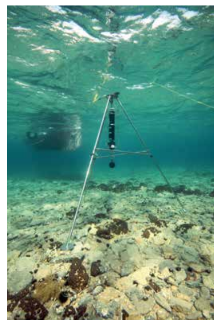
Fig. 6.2 Side scan sonar image (400 kHz), obtained in 2-4 m water depth of the submerged prehistoric city of Pavlopetri in Greece. Blue lines highlight the remains of the walls of the buildings and roads. (Sakellariou et al. , 2011) The image on the right shows a sector-scanner (Kongsberg MS1000) mounted on a tripod, and deployed in the centre of the ruins at Pavlopetri. The sector scanner projects sound at 750 kHz, and rotates in the tripod to build up a radial picture.
