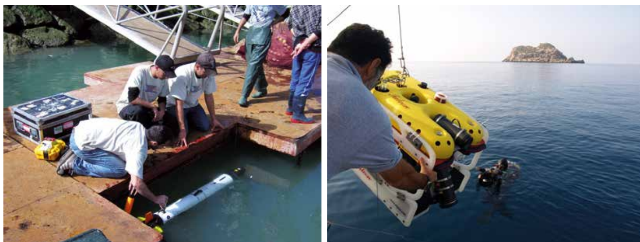
Fig. 6.9 Launching of an Autonomous Underwater Vehicle (AUV, left) and Remotely Operated Vehicle (ROV, right) for underwater archaeological surveys.
