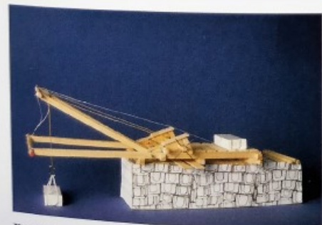
Fig. 51a-e — Reconstruction of the machinery used for placing the blocks (CAD EFA, T. Koželj)
