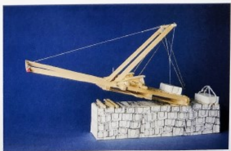
Fig. 51a-e — Reconstruction of the machinery used for placing the blocks (CAD EFA, T. Koželj)
