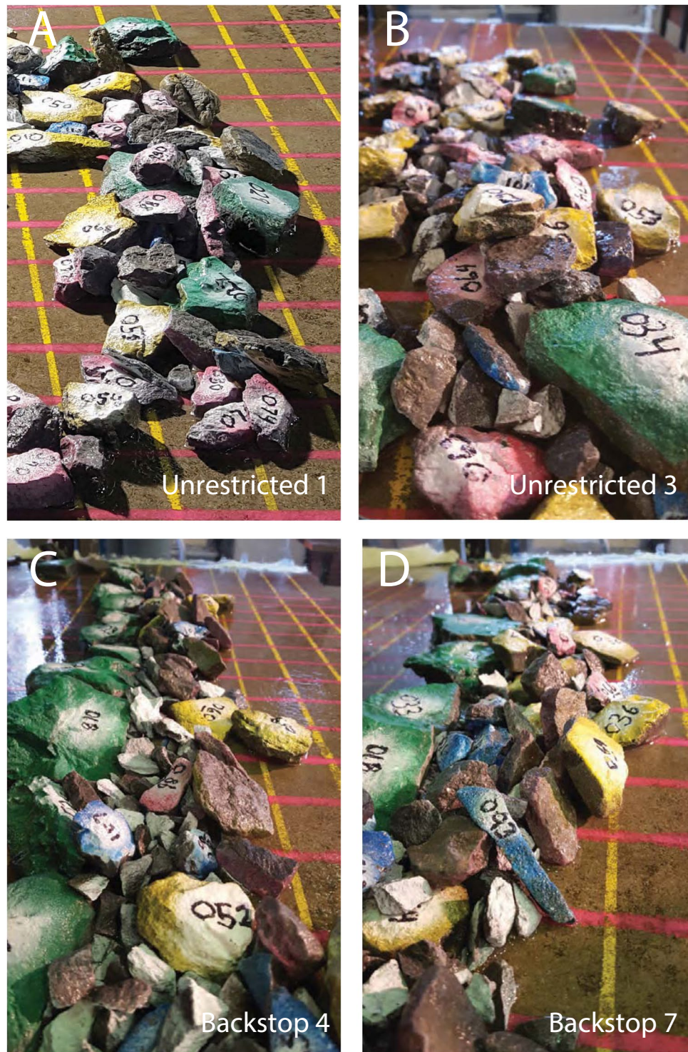
Figure 6. Patterns of stacking and imbrication from several different tests. The specific tests (see Table 1) are indicated on each image. (A,B) Show unrestricted platforms and (C,D) show backstopped platforms. Grid spacing is 5 cm (=5 m at full scale), and clast colours and numbers are keyed to Supplementary Table S1.
