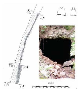
Fig. 10. Bucium: photo, overall plan and section cuts in the Roman gallery at "Baia Domnilor" (former "Petru şi Pavel") mine.
