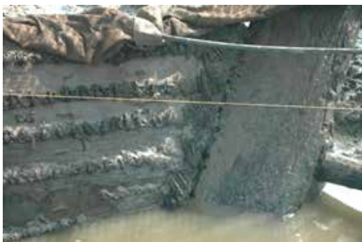
Figure 4.9 Excavated sternpost (or stempost) section and planks of the Phanom Surin ship illustrate the surviving sewing ropes stitched over the wadding to seal the joinery
