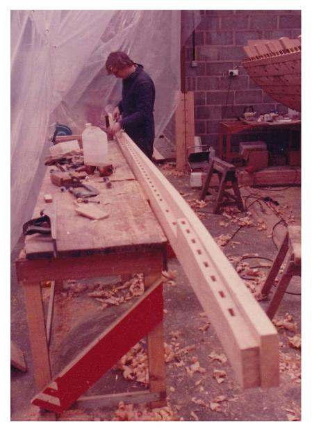
*Fig.* 3.2. The ancient shell-first method of ship construction. A shipwright cutting mortice holes into a garboard on a trial section of a replicated Classical trireme. Picture courtesy of Malcolm Adkins.
