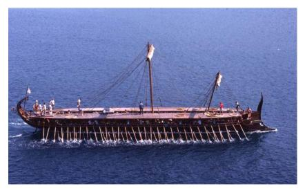
*Fig.* 3.9. The replicated trireme *Olympias* under oars during sea-trials off Poros in 1988. Photo: Courtesy of The Trireme Trust.
