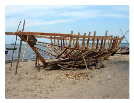
*Fig.* 3.1. A traditional wooden 'skeleton-first' fishing boat being built on the beach at Petite-Anse in Cap-Haitien, Haiti. As can be clearly seen, the frame or 'skeleton' of the vessel is erected first. Once in position, the planking of the hull is then nailed directly to the ribs of the vessel. Photo: Rémi Kaupp.
