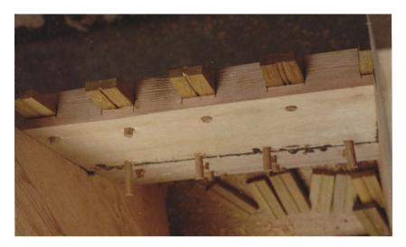
*Fig.* 3.3. Shell-first ship construction. Trial section of a replicated Classical trireme depicting tenons positioned in their mortice holes below and awaiting to be guided into those of the planking above. Hardwood pegs, which provide additional strength to the mortice-and-tenons, can also be seen, locking the tenons in place. Picture courtesy of Malcolm Adkins.
