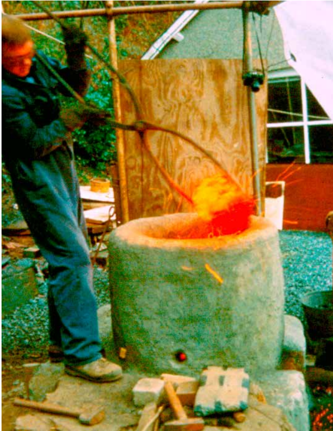
Figure 1 Experimental iron working at Plas Tan y Bwlch, Gwynedd: removing a bloom from a furnace. [photo © David Starley]
