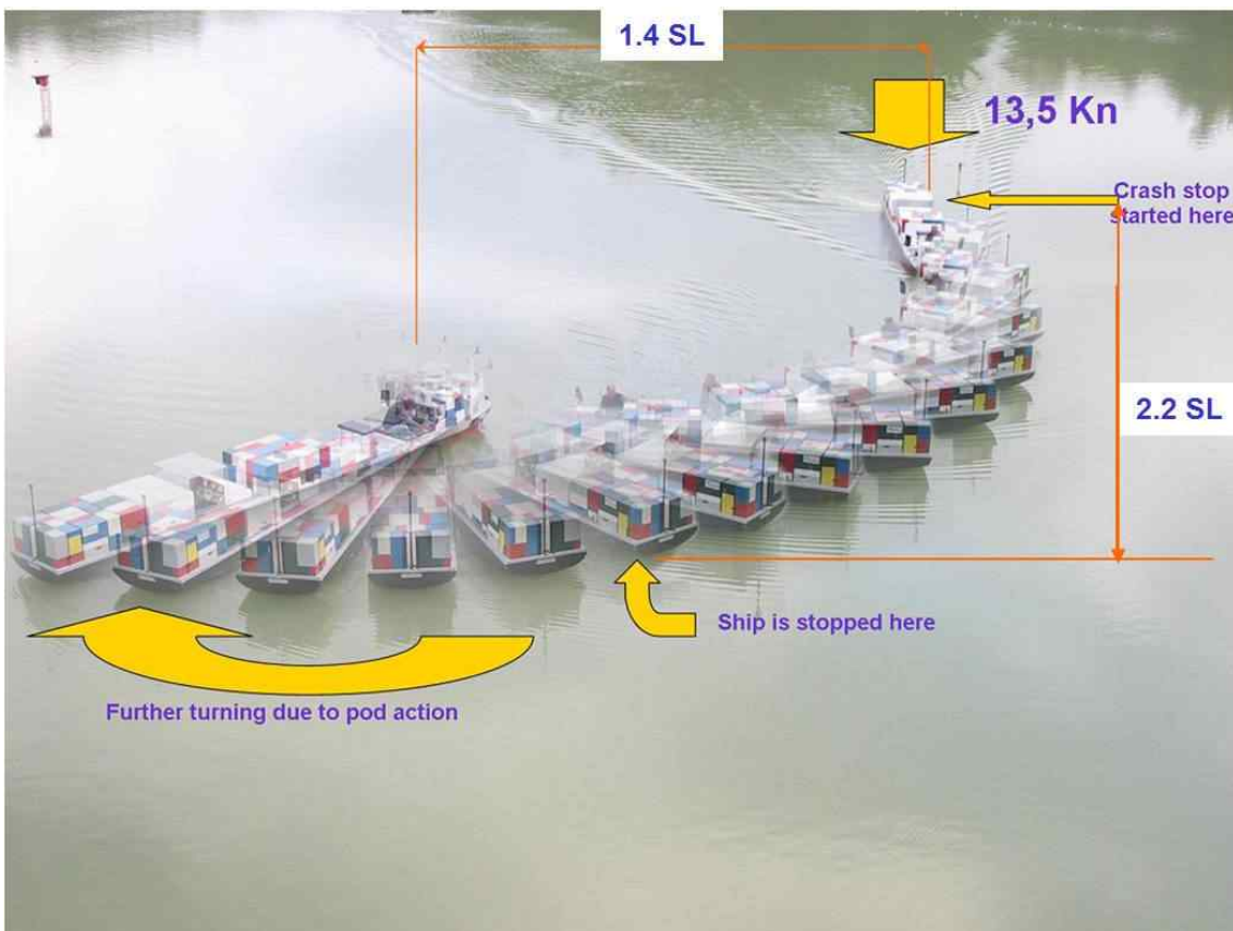
Crash stop by turning the ship. With an initial speed of 13.5 knots, the ship is stopped in 120 seconds, in an area equivalent to only 2.2 x 1.4 times its length.
