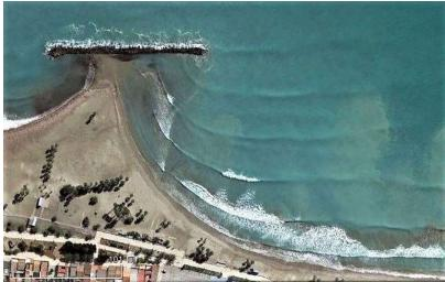
Wave diffraction pattern behind a detached breakwater Xilxes, Spain (Google Earth, 2015)
