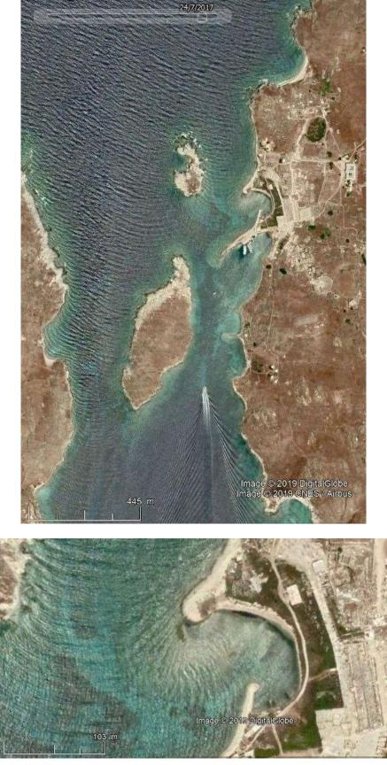
Wave pattern in Delos Channel with mild northern Meltem wind (Google Earth 24/7/2017) showing fair shelter in Sacred Port thanks to Lesser Remmatia islet and remains of northern "large mole". See also wave diffraction pattern around the remains of the large mole. The remains of the large mole were surveyed by Philippe Fraisse at the end of the 20<sup>th</sup> c.
