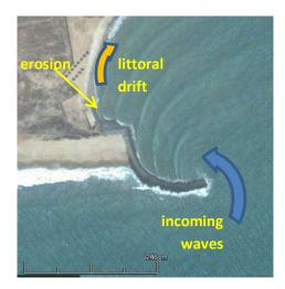
Waves diffracting around the breakwater head, inducing erosion at the breakwater landward end (Cotonou, Benin)
