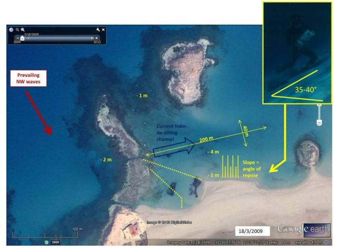
De-silting current from Channel 2
