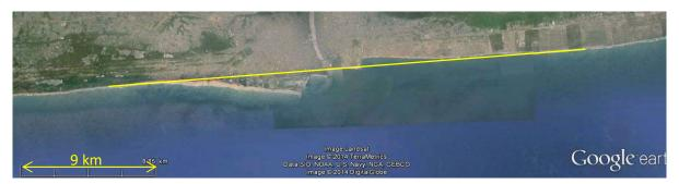
This picture shows the initial shoreline near Cotonou (Benin) (straight yellow line). This was the shoreline before any human construction (a port) was built in the sixties. This coast is known for its littoral drift of around one million cubic meters per year from west to east (left to right on the picture).
